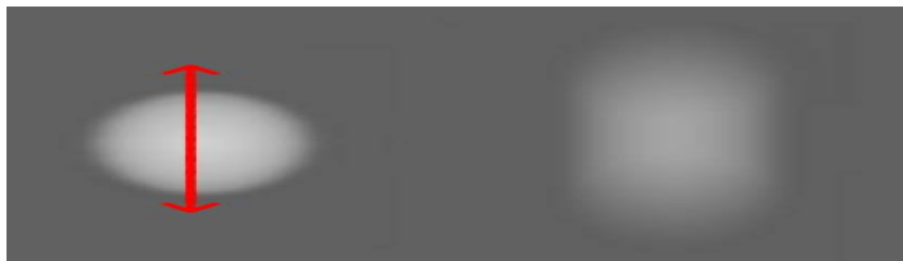
Figure 2: An example of blurring (right) resulting from the vertical motion of an object (left)
